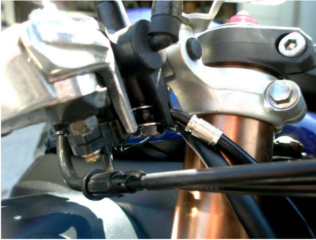
a. Front master cylinder, notice position and sequence
