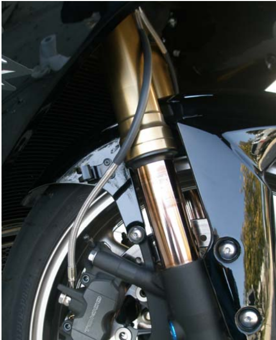
c. Right caliper, lines routed in front of the forks
