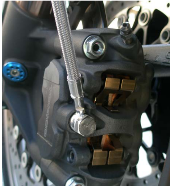
f. Left caliper, notice positioning of fitting
