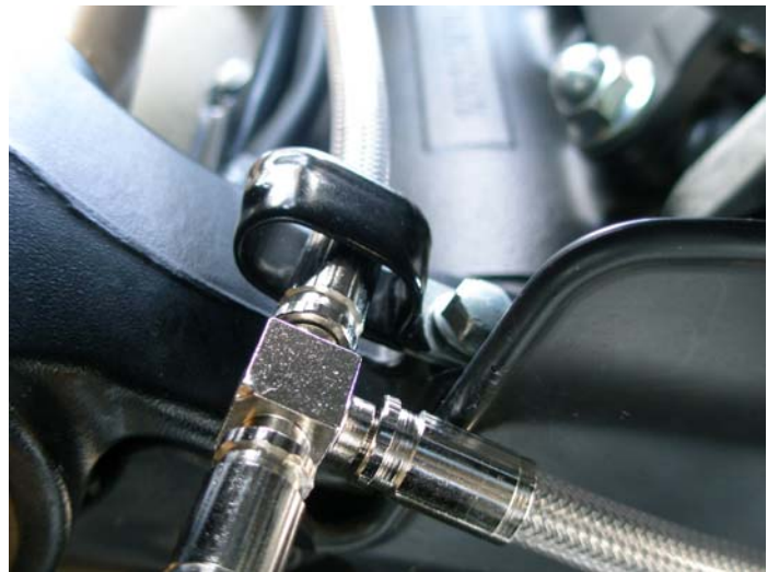
b. Top line routed through Galfer c-clip at lower triple tree
